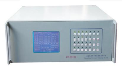
Portable power source of program control is for site production line. With the technology of PWM pulse width modulation amplifier, the equipment offers the features of large output power, high stability, low power consumption, high efficiency and small size. Providing stable and ideal operation condition for measurement of 50Hz operating frequency, the equipment is suitable for all kinds of energy meters.
