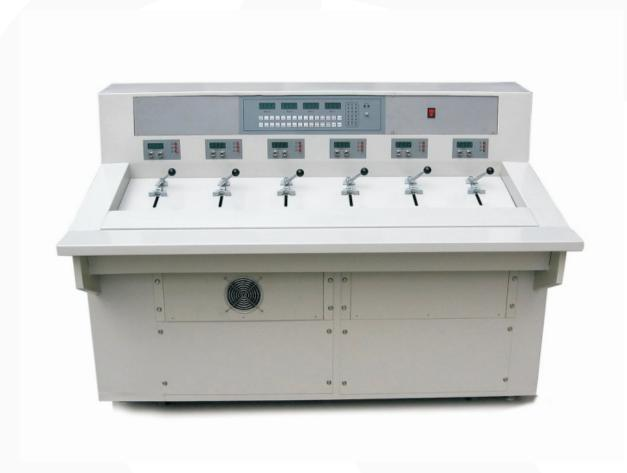
The bench is small size plane test equipment, which is specially designed according to single-phase meter's calibration features. The operating theory is the same as that of single-phase meter test equipment. From the structure, it is convenient to solder. Resistance will not slide down when meter is on test bench flatly. Thanks to small size, the bench can stay at both sides of production line as one part of production line.
