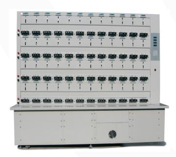
With PWM modulation amplifier, the equipment offers large power output, high reliability and stability.
